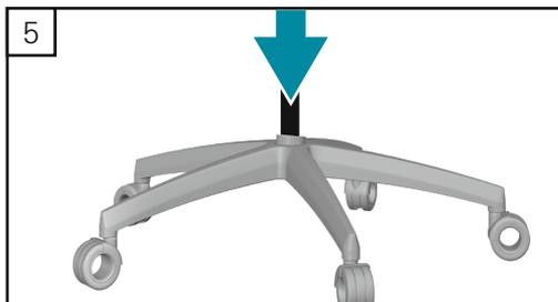
3. Put the upper end of the gas spring into the mechanics module. Then tilt the complete seat back into an upright position and place it on the castors. [6]
